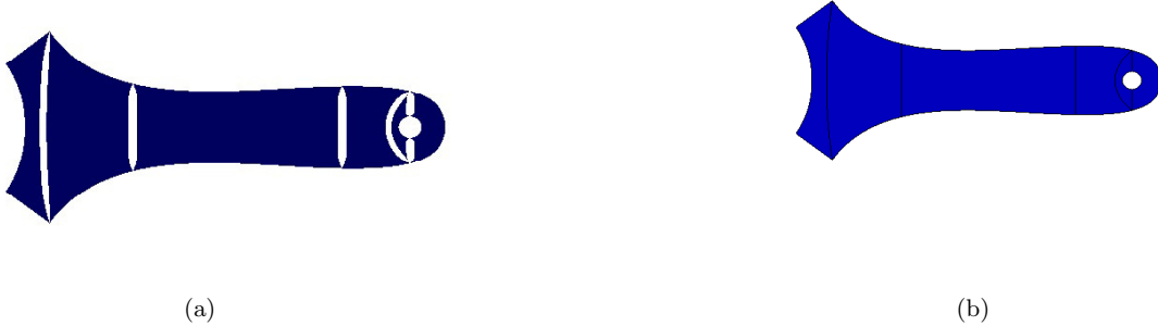
Fig. 1. (a) A geometric illustration of a decomposition including gap regions between the adjacent subdomains, (b) The decomposition without any gap region.
